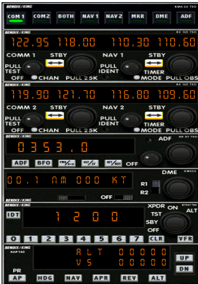
Fig. 6. Microsoft Flight Simulator 2004's generic radio stack. It is modeled after Bendix/King Silver avionics system.
