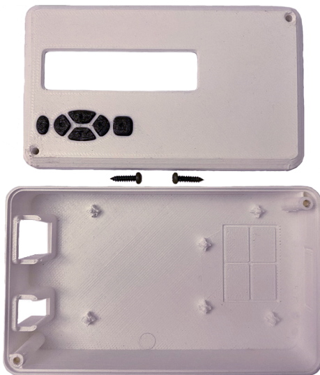
Fig. 9. 3D printed case to accommodate an Arduino with a LCD Keypad shield connected
