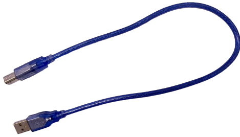
Fig. 8. USB type B to USB type A cable for the communication between the Arduino board and the computer.
